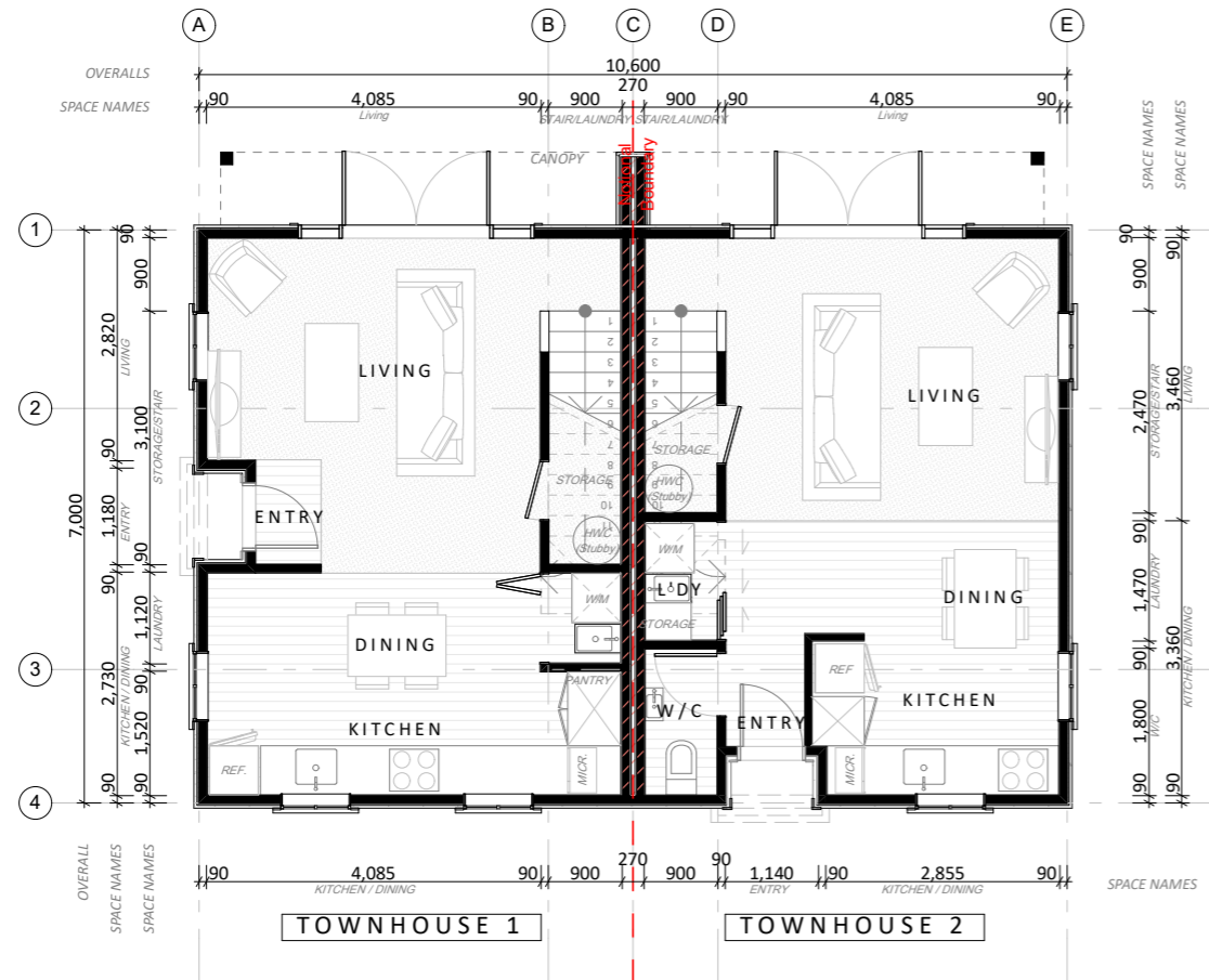
1. GROUND FLOOR PLAN SCALE 1:100
