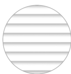
Cladding - Timber Weatherboard
